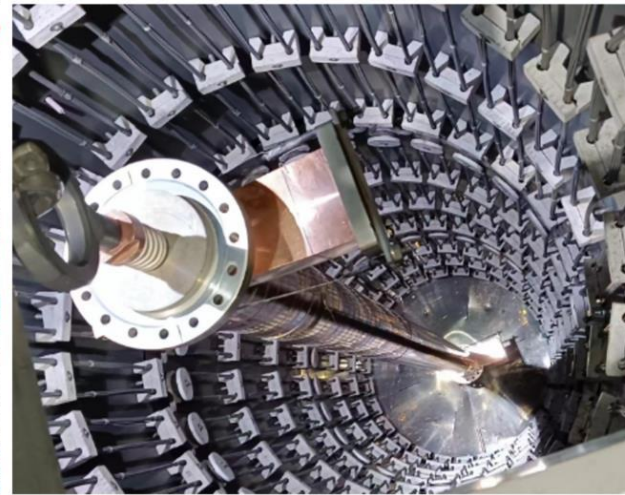
Brazing in vacuum or hydrogen furnace using different alloys at different temperatures (650-850 C) and/or in different steps
