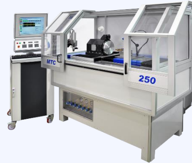
Precision turning of cells, surface roughness < 50 nm, precisions of the order of few \mu\text{m}
