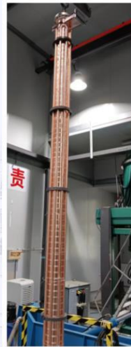
Brazing in vacuum or hydrogen furnace using different alloys at different temperatures (650-850 C) and/or in different steps
