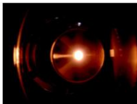
Thermionic gun with \phi 3mm CeB 6 cathode
