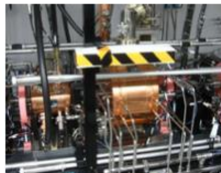
476 MHz booster cavity + L-band correction cavity
