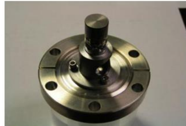
a typical type B dispenser cathode for linac system
