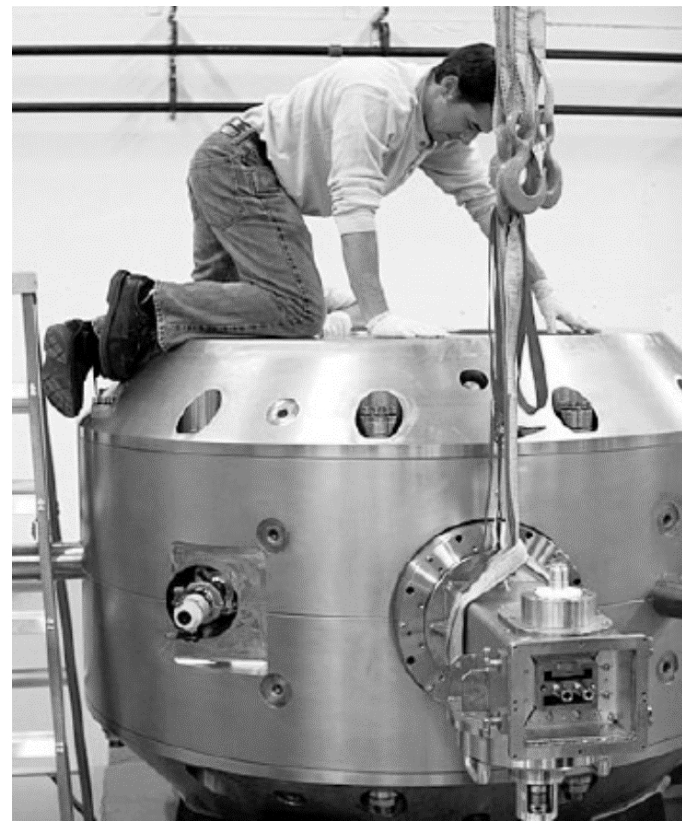
Mevion S250 with SC magnet B=9T (20 tons)
