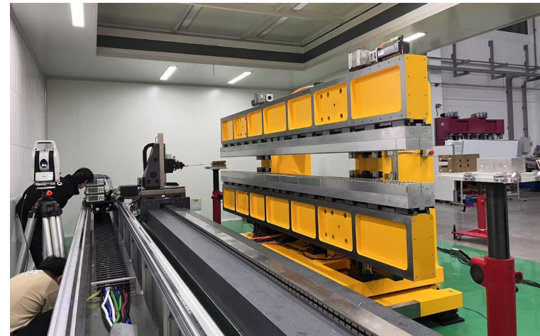
Fiducilisation of the magnetic center of undulator
