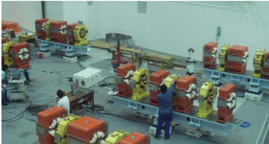
Pre_alignment of the magnet and vacuum chamber
