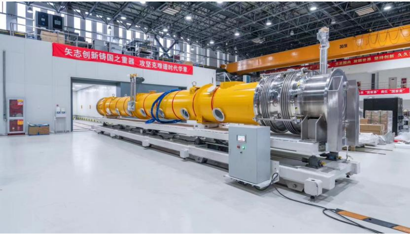
The first high Q high gradient performance medium-temperature baking 1.3GHz cryomodule
