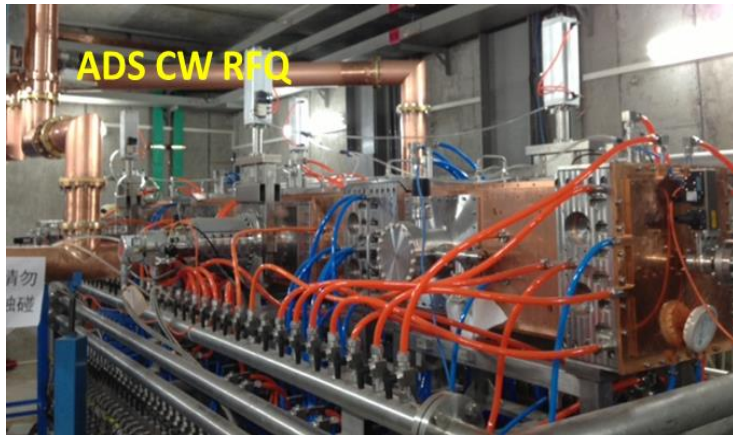
2.1 MeV/H + 10 mA, 2011-2014, 3 such RFQs were built and being operated at IMP
