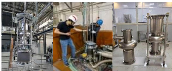
Vertical Testing of the RF Cavity
