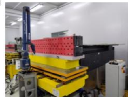
Measuring BLG magnet with Arm based planar moving coil system
