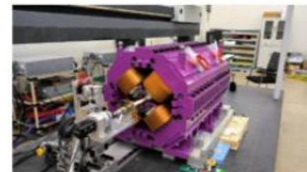
Measuring BD magnet with CMM based Rotating coil system
