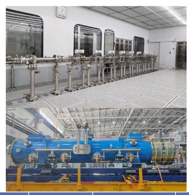
Nineteen 3.9GHz cavities, fabricated by OSTEC, surface treated at Wuxi platform. tested in Shanghai
