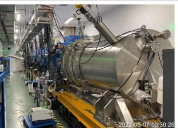
CM prototype with 8 BCPed cavities
