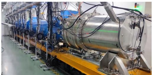
CM prototype with 8 high-Q cavities
