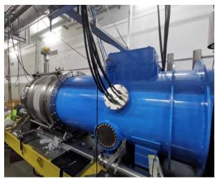
Test CM for 1.3/3.9GHz single cavity
