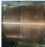
3m-long absorber in electron beam welding
