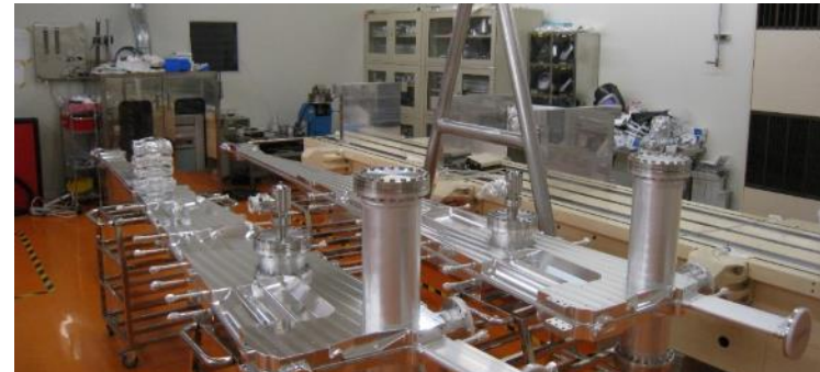
Large Aluminum Alloy Vacuum Chamber with Ultra-Low Outgassing Rate (NSRRC)
