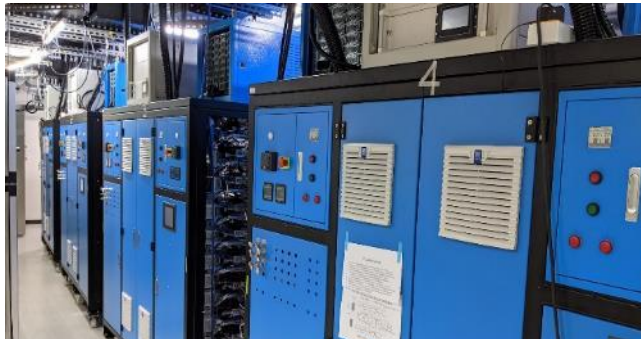
320 kW 500 MHz High-Power Solid-State RF Source (NSRRC)
