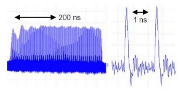
Figure 7: Multi bunch mode WCM2 trace: Entire pulse train (left) and detail (right).
