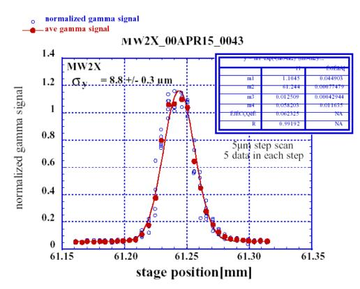
(left) wire scanner chamber installed in the ATF (KEK) extraction line and (right) example wire scan (courtesy H. Hayano, 2003)
