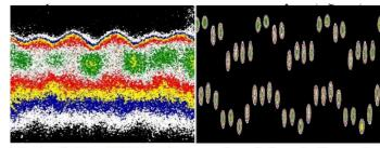
Fig.3a (left) : ESRF at low  $\alpha$  : bunch length fluctuation Fig. 3b (right) : ESRF HOMs causing longit. instabilities
