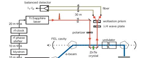
Electro-Optic Technique with Improved Time Resolution for Real-Time, Nondestructive, Single-Shot Measurements of Femtosecond Electron Bunch Profiles -PRL2004
