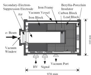
cross-sectional view of the FC of the KEKB injector linac (courtesy T. Suwada, 2003)
