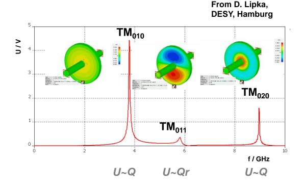
When the particle bunches pass through the resonant cavity, it excites multiple electromagnetic modes:
